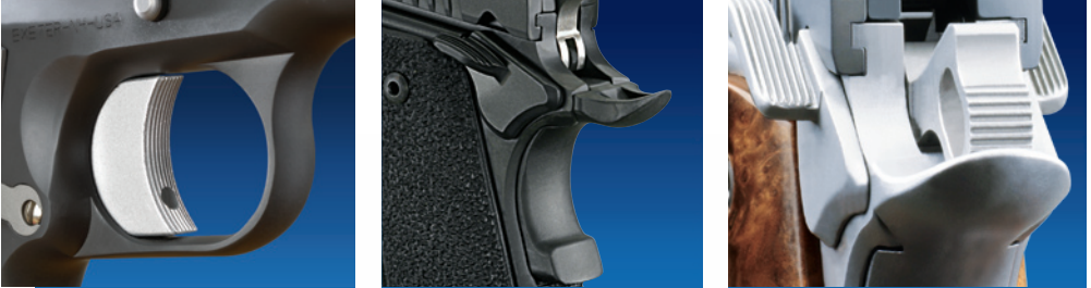
The 1911 features a lightweight aluminum match trigger, raised grip safety for sure deactivation, and a speed hammer to shorten lock time.
